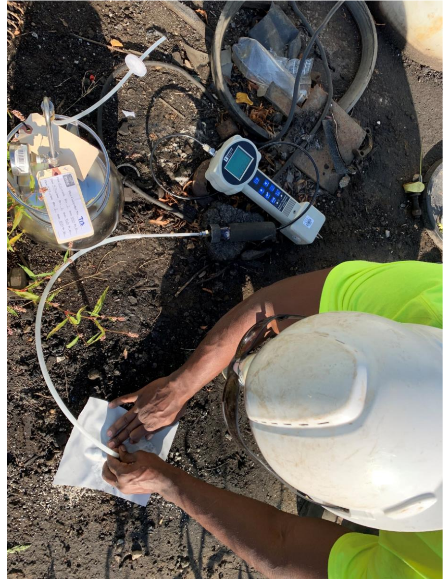
Helium test prior to soil vapor testing
