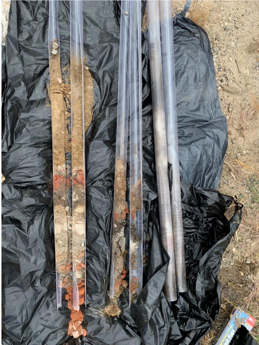
Soil boring depicting historic fill
