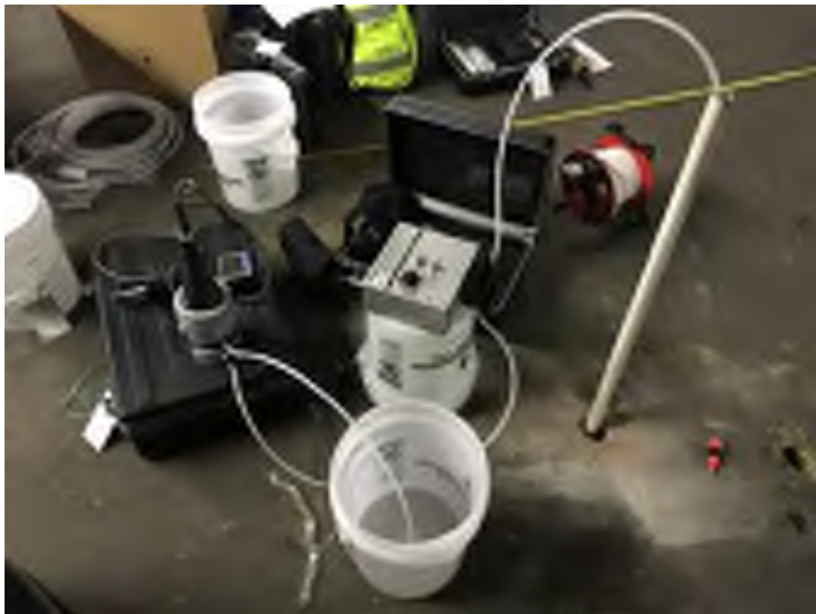
Photo 6: View of groundwater purging and sampling setup. (facing west)
